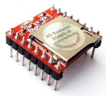
The SOMO-II features an on board 16bit MCU, specifically designed for hardware audio decoding.
