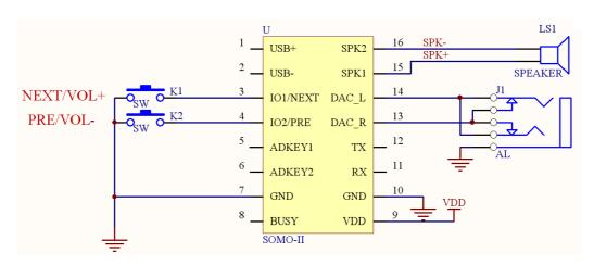
This is an example schematic showing the simplest connections to the SOMO-II for KEY MODE. Only 2 buttons are required. NEXT/VOL+ will start playing a track if currently stopped, and will raise the volume if the button is held down for > 1.2 seconds. PRE/VOL- will start playing a track if currently stopped also, and will lower the volume if the button is held down for > 1.2 seconds. See the table in Section 5.3 for more information.
