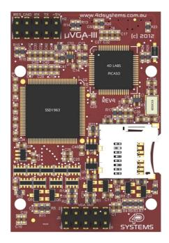
The **micro-SD** card slot provides the user with expandable memory space suitable for multimedia file retrieval, including images, animations and movie clips, as well as data logging applications.
