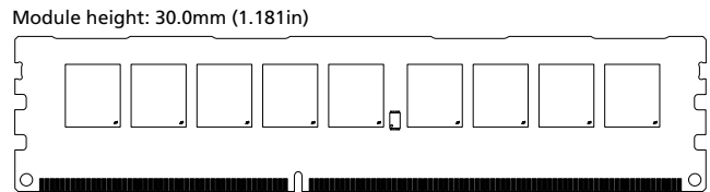
Figure 2: 240-Pin UDIMM (MO-269, PCB 1561 R/C E3)
