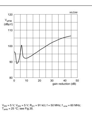
Fig.12 Unwanted voltage for 1% cross-modulation as a function of gain reduction; typical values; amplifier a.
