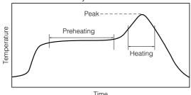
For soldering (Example: Sn/Pb)
