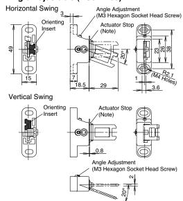
Actuator Mounting Hole Layout (horizontal/vertical swing)
