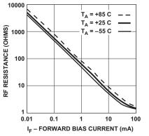
Figure 2. RF Resistance vs. Forward Bias Current, f = 100MHz
