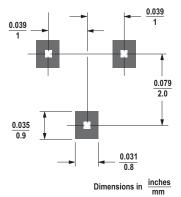
Figure 13. Recommended PCB Pad Layout for Avago's SOT-23 Products.
