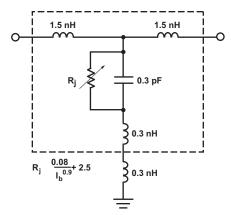
Figure 9. Equivalent Circuit.
