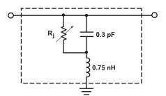
Figure 11. Equivalent Circuit.
