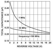
Figure 1. RF Capacitance vs. Reverse Bias.
