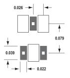
Dimensions in inches Figure 12. Recommended PCB Pad Layout for Avago's SC70 3L/S0T-323 Products.
