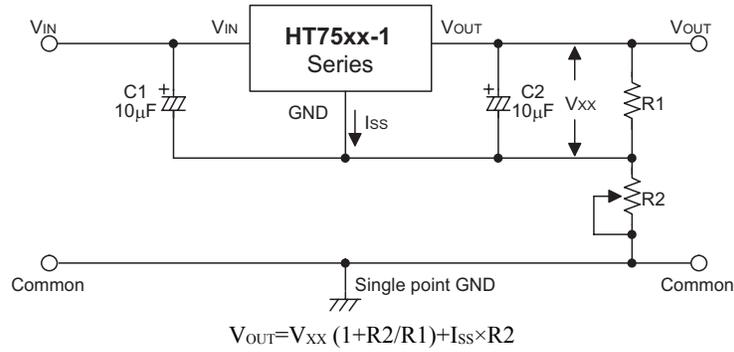
**Circuit for Increasing Output Voltage**
