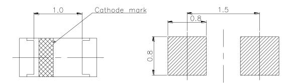
**Note:** The tolerances unless mentioned are  $\pm 0.1$ mm, unit = mm.
