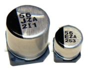
Rated for 105°C, type HZA combines the advantages of aluminum electrolytic and aluminum polymer technology. These hybrid capacitors have the ultra-low ESR characteristics of conductive aluminum polymer capacitors packaged in a V-chip, SMT case with high capacitance and voltage ratings
