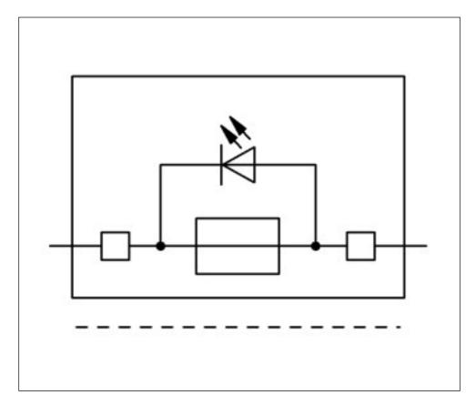
Printview: Fuse plug with pull-tab; for 5 x 20 mm miniature metric fuse; with indicator lamp; 12 - 30 V; 7.4
