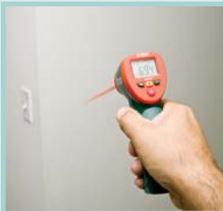
Check building for insufficient insulation
