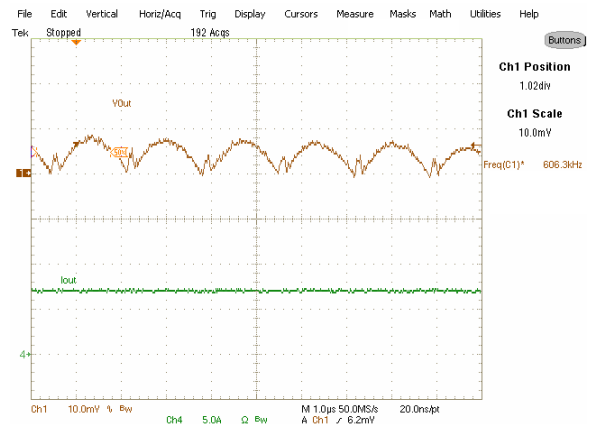
Fig. 10: Output Voltage Ripple, 7A load, V_p: 0.6V , Ch_1: V_{out} , Ch_4: I_{out}
