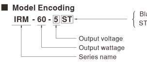
Blank : PCB mounting style ST : Screw terminal style
