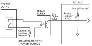
Note: When energized (switch in the "on" position), a low load terminal voltage will be present when fuses are open or when pullout module is removed. The leakage current is limited to .5mA maximum.
