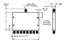
All dimensions are ± .020, except mounting hole diameters (± .005) and mounting hole location ( $\pm$  .010) .
