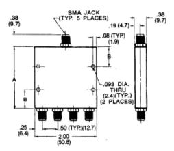
Note: All dimensions are  $\pm$  .020, except mounting hole diameters  $(\pm \ .005)$  and mounting hole location  $(\pm \ .010)$  .
