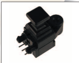
OTJ-1/ORJ-1 Single Optical Transmitter and Receiver Jack. Right angle PCB mount with self tapping hole for panel mounting. Removable plug-in cover.
