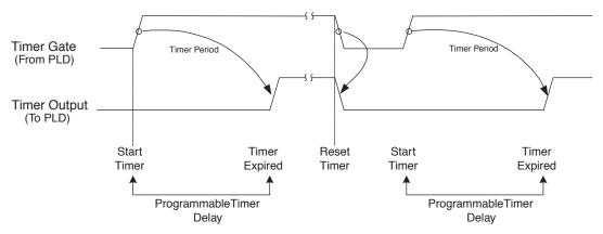
Note that if the clock module is configured as "slave" (i.e. the CLK is an input), the actual time-out of the two timers is determined by the external clock frequency.
