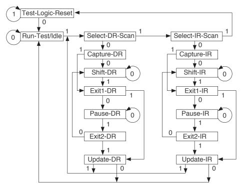
Note: The value shown adjacent to each state transition represents the signal present at TMS at the time of a rising edge at TCK.
