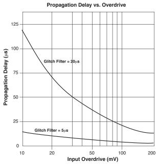
Note: Typical propagation delay of  $V_{MON}$  inputs to outputs as a function of overdrive beyond selected trip point.
