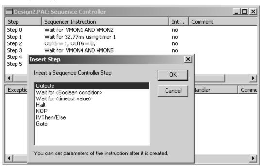
Programming of the ispPAC-POWR604 is accomplished using the Lattice ispDOWNLOAD Cable. This cable connects to the parallel port of a PC and is driven through the PAC-Designer software. The software controls the JTAG TAP interface and shifts in the JEDEC data bits that set the configuration of all the analog and digital circuitry that the user has defined during the design process.
