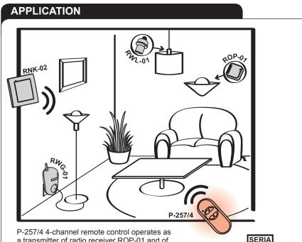
P-257/4 4-channel remote control operates as a transmitter of radio receiver ROP-01 and of remote control socket RWG-01. RNK-02 radio button transmitter and RWL-01 radio lighting switch are also devices of EXTA FREE system.
