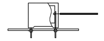
Temperature monitored inside the capacitor.
