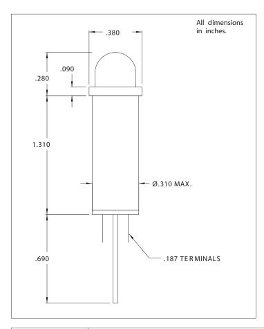
Solid-state indicator lights complete with built-in current-limiting resistor and rectifier diode.
