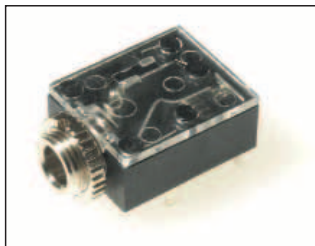
JYS-35 stereo switched 3.5mm Jack Socket. Right angle PCB mounting. Supplied with ring nut.
