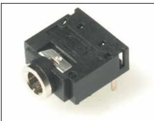
JYO-39-3P stereo unswitched 3.5mm Jack Socket. JYO-39-5P stereo switched version. Right angle PCB mounting.
