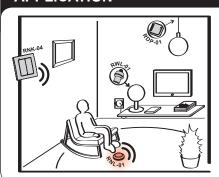
Radio foot transmitter RNL-01 controls operation of RWL-01 radio lighting switch (switch on / switch off) or RDP-01 radio dimmer (switch on / switch off, light brightening / dimming). The receivers can be controlled by 4-channel button radio transmitter RNK-04. The RNL-02 transmitter does not require additional installation, external power supply connection
