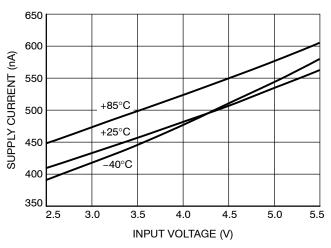
Figure 2. Supply Current vs. Input Voltage
