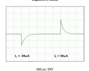
Figure 10. Load Transient Response
