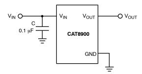
Figure 1. Application Circuit
