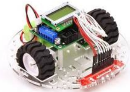
Pololu 5" round robot chassis RRC04A with an Orangutan SV-328 and a QTR sensor array.
