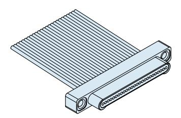
**Glenair Insulated Wire Nano Connectors** feature gold alloy TwistPin contacts. Contacts are precision-crimped to insulated, stranded wire. These nanomimiature connectors offer premium performance and reliability for demanding applications. Contact spacing is .025 inches. 1 amp current rating, DWV rating 250 volts AC. Wire gages #30 and #32 AWG.
