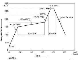
NOTES: 1.We recommend the reflow temperature 245°C(+/-5°C).The maximum soldering temperature should be limited to 260°C. 2.Don't cause stress to the epoxy resin while it is exposed to bit temperature to high temperature. 3.Number of reflow process shall be 2 times or less.
