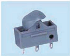
RSM1026 ON-ON 12 A 125 VAC; 6 A 250 VAC SPDT 3P
