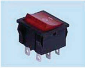
RSM2024 ON-ON 10 A 125 VAC; 6 A 250 VAC DPDT 6P
