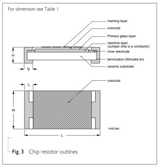
Chip Resistor Surface Mount RV series 0805/1206/2512 (RoHS Compliant)
