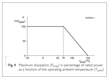
Chip Resistor Surface Mount RV SERIES 0805/1206/2512 (RoHS Compliant)
