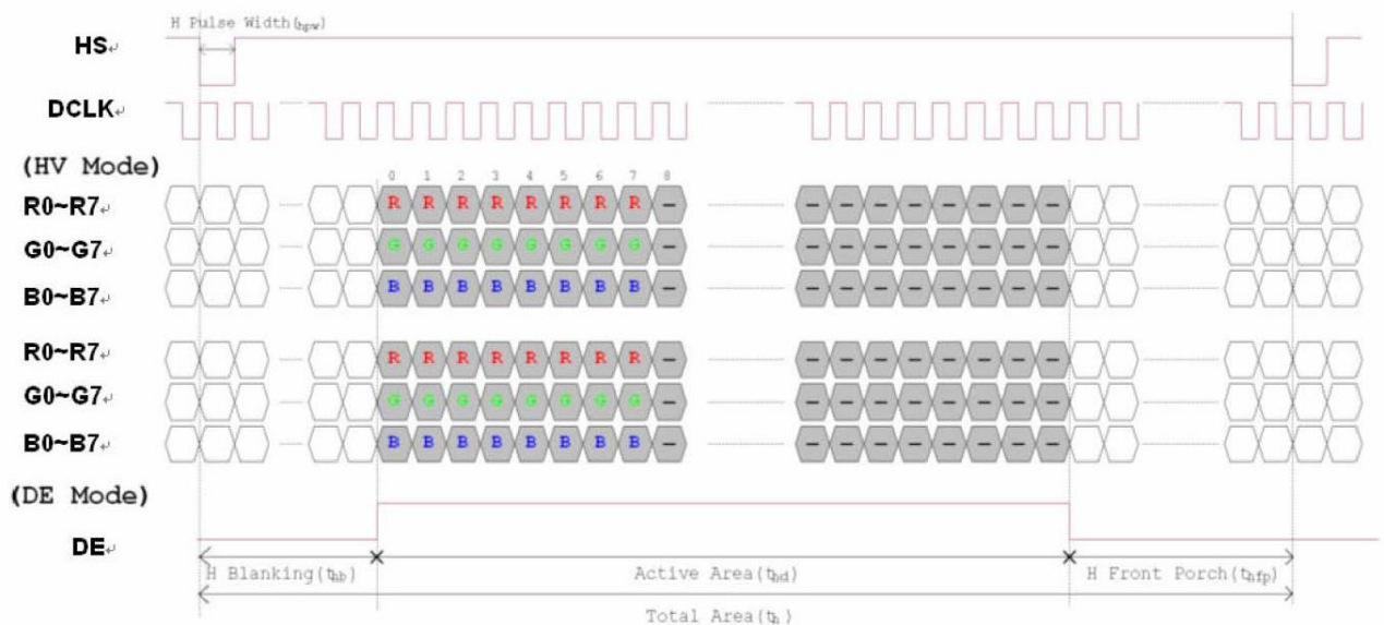
Figure 7. Horizontal input timing diagram
