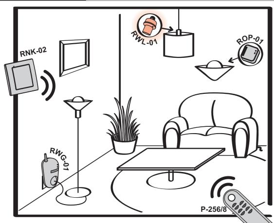
Radio lighting switch RWL-01 operates as a receiver of 8-channel remote controller P-256/8 and of 2-channel button radio transmitter RNK-02 (switch on/switch off control of a light source installed in E27 thread in RWL-01 device). The above mentioned transmitters can also control operation of 1-channel flush receiver ROP-01 and of remote control socket RWG-01.
