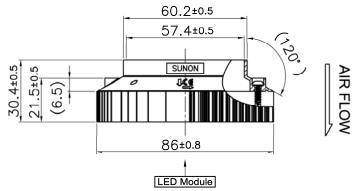
Assembly direction of customer's LED Module
