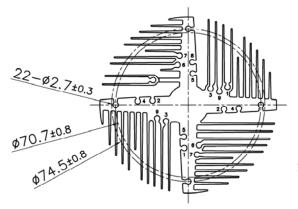
For LED Module Assembly Screw torque max 12kgf.cm
