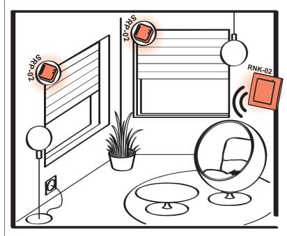
Radio flush dimmer RNK-02 operating roller blind controller SRP-02 (roller blind opening / closing). The above mentioned transmitter can be added to any number of receivers.
