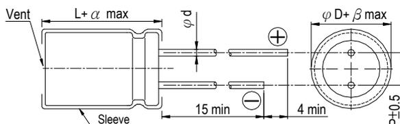
Dimension:  $\phi D \times L(\text{mm})$
