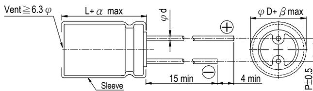
Lead Spacing and Diameter Unit: mm
