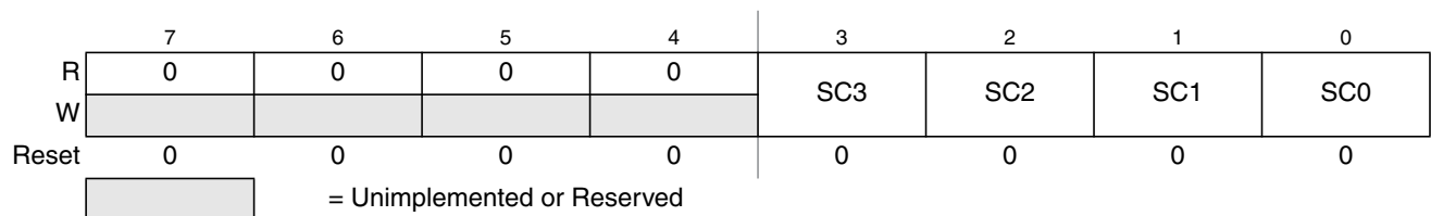
Figure 8-9. Debug State Control Register 1 (DBGSCR1)
