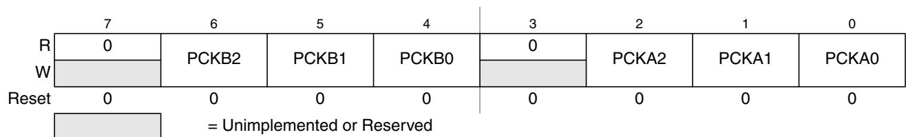
Figure 17-6. PWM Prescale Clock Select Register (PWMPRCLK)
