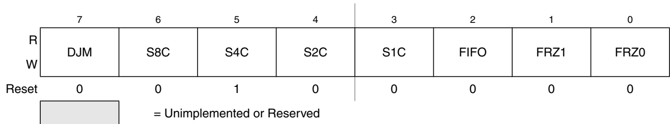
Figure 11-6. ATD Control Register 3 (ATDCTL3)
