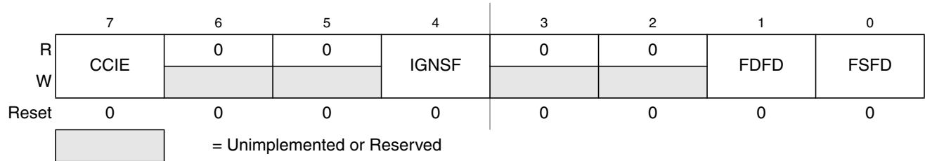
Figure 24-9. Flash Configuration Register (FCNFG)
