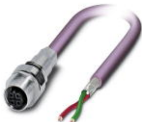
Bus system flush-type socket, PROFIBUS, 2-pos., M12, shielded, B-coded, front/screw mounting with M16 thread, with 0.5 m bus cable, 2 x 0.25 mm 2
