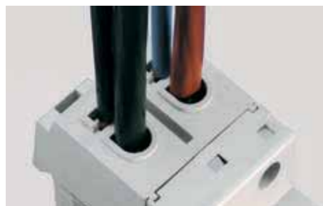
Without busbars two terminal spaces can be used for cables with different cross sections: incoming supply with supplementary terminal up to 50 mm 2 from the front side.
