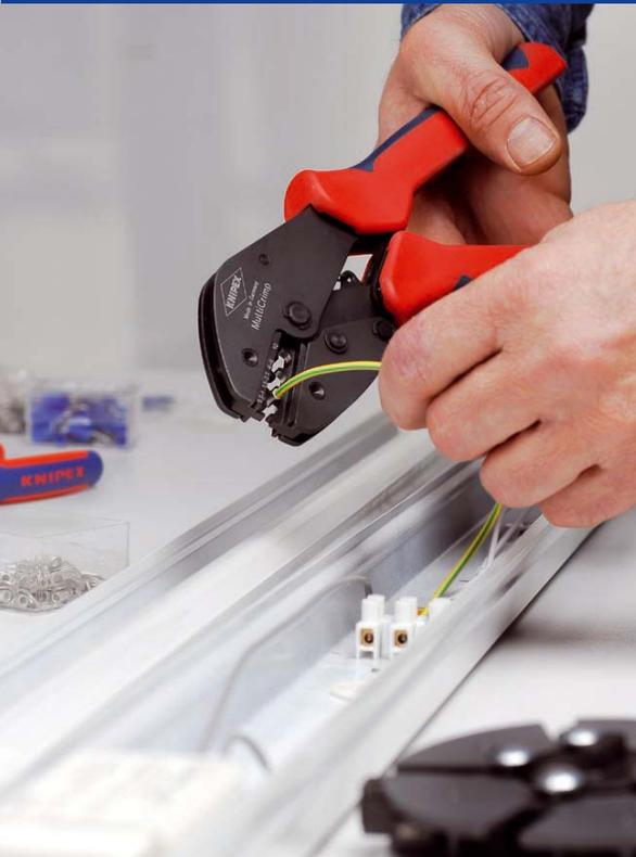
The electrician travelling in mobile services needs at least 3 different crimping pliers to be prepared for crimping of the most common standard connectors. The new MultiCrimp system now offers the compact solution for the professional user: a set of optionally 3 or 5 interchangeable crimping dies in a quick changer magazine for the most common applications on the spot.
