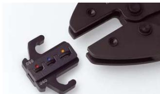
Catch for exchange of crimping dies
