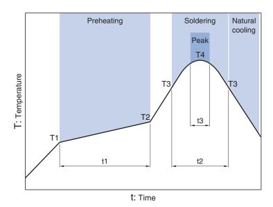
Soldering Preheating Peak Time Time Temp. Time Temp. Temp. T2 **T3 T4** t3 150°C 180°C 60 to 120s 230°C 30s 250°C 5s
