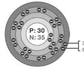
2 electrons on outer layer are given up by the zinc atoms
