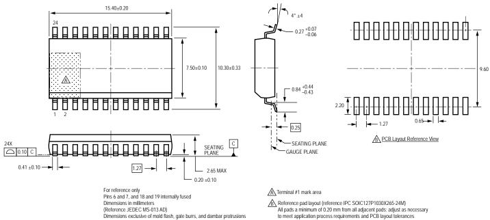
Dimensions exclusive of mold flash, gate burrs, and dambar protrusions Exact case and lead configuration at supplier discretion within limits shown
