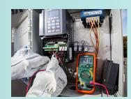
These professional DMMs are loaded with advanced features and functions. Low Impedance (LoZ) mode eliminates false readings caused by ghost voltages. Low Pass Filter (LPF)attenuates high frequencies to reduce noise for accurate readings. True RMS provides accurate readings when measuring distorted or noisy waveforms. Built-in Non-Contact AC Voltage Detector quickly checks for the presence of AC Voltage before testing.
