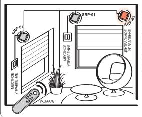
Roller blinds control system realised by means of wired roller blind controllers SRP-01. One controller can be used for one roller blind. Each of the controllers has a local control push-button and connected inputs of central control. which allow to close or open a given group of roller blinds by means of SRP-03 device - central roller blinds controller. SRP-03 is operated in a wireless way by means of 8-channel remote control P-256/8. Roller blinds switches can not be equipped with backlight.
