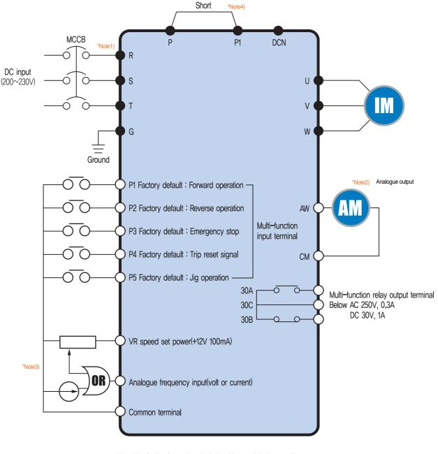
\*Note1)" "and" "means the main circuit and the control circuit respectably. Please connect to the R and S terminals in case of single phase use.
