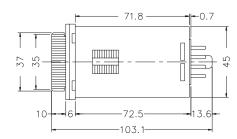
Y type(Flush Mounting): Using Y50 Frame & US-08 Socket or P3G-08 Socket
