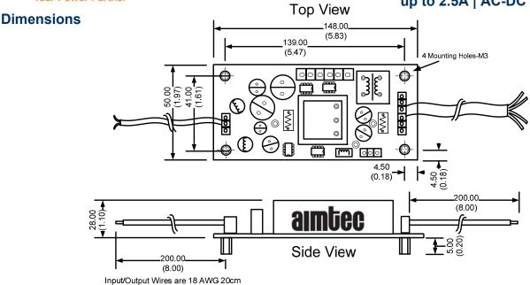
**NOTE:** to adjust the output current connect a 20K Ohm pot between blue and white wire
