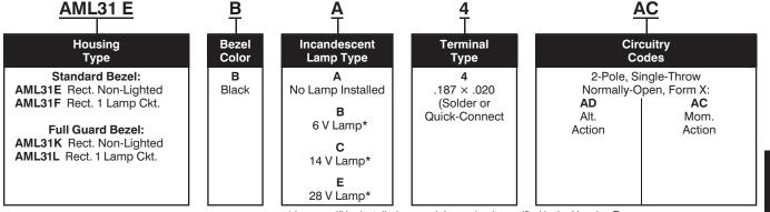
\* Lamps will be installed per each lamp circuit specified in the Housing Type.
