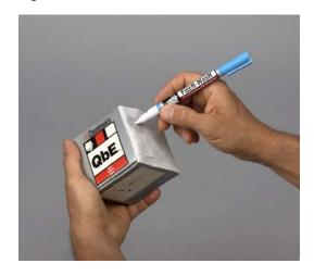
[7] When moistening a precision swab for back plane cleaning, hold the swab tip in the 1" spot of cleaner for a count of 1-2-3-4-5 (about 5 seconds). Insert the swab and rotate the hand three times. Follow up with a dry swab.
