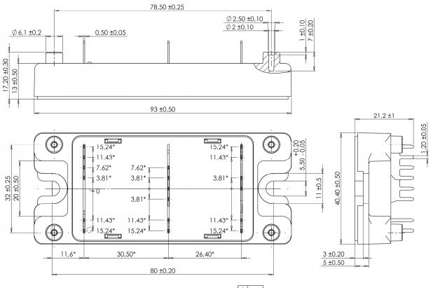
All dimensions marked "\*" are toleranced as :  $\phi$  Ø 1
