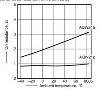
2.-(2) On resistance vs. ambient temperature characteristics
